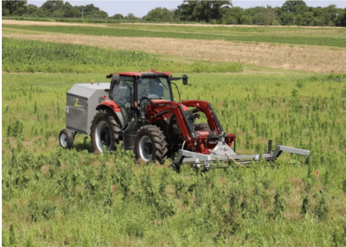
Missouri researchers used a Case IH tractor to pull the Weed Zapper, which supplies electricity to a copper bar mounted on the front. Photo credit: University of Missouri Weed Science
