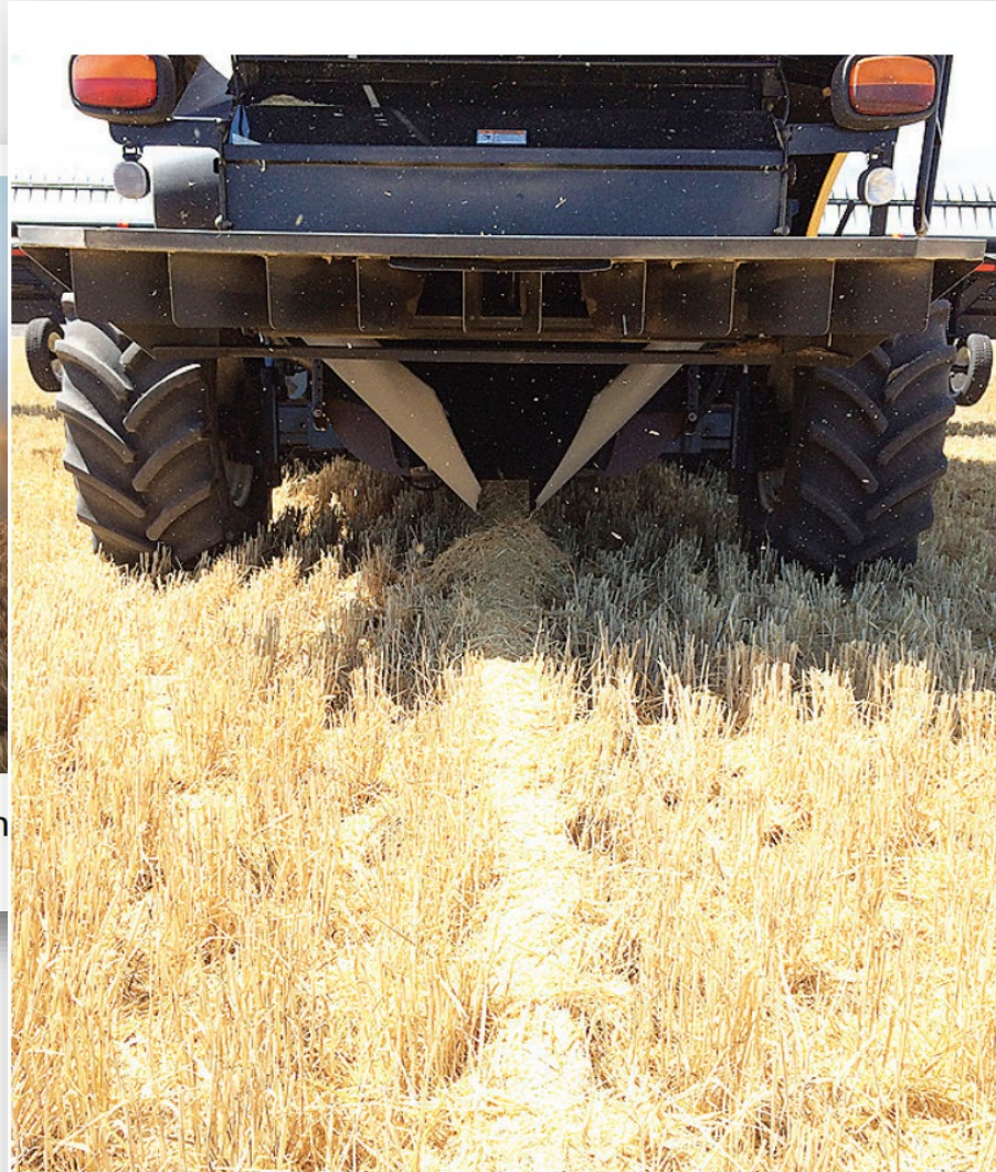
FIGURE 41 The Mic Fels-designed New Holland chaff line chute in action.
